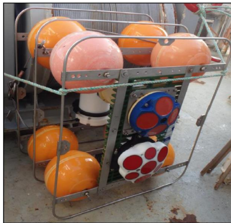
Figure 2: On the front, the two ADCPs used for the tests mounted on the raft
