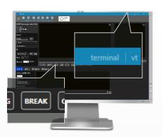
Open Pulse, go to TERMINAL in top right corner. Set the serial port and baud rate. By default the ADCP is 115200 8N1. Then click the BREAK button to verify communication.
